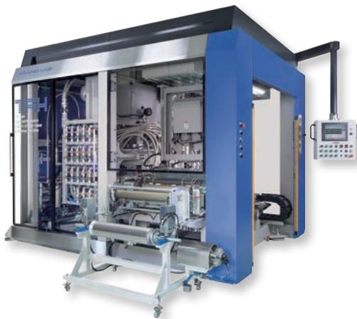
"3D Surface decorative forming" utilizing thermoforming technology is the method to add the value to the surface of base material (for instance, injection molded parts) by covering and adhering the high level of sheet like with decoration.
