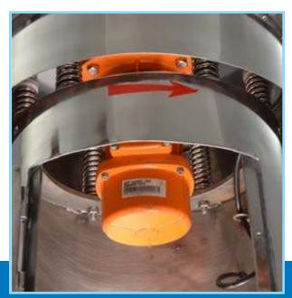
**Eccentric Motor for Controlled Vibration**
