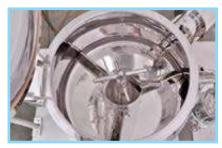
Specially designed Radial Impeller
